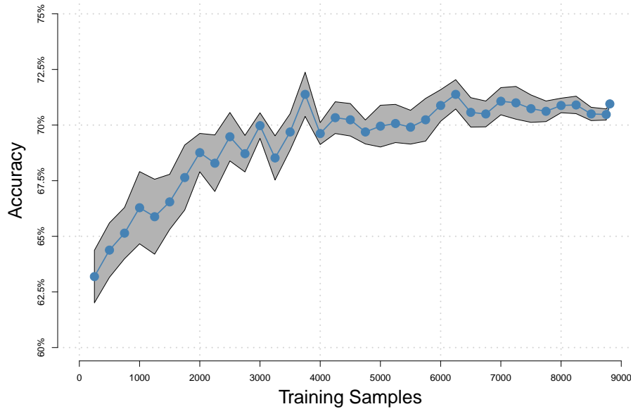
Figure 3: Accuracy of the Baseline Machine Learning Classifier as a Function of Size of the Training Dataset
